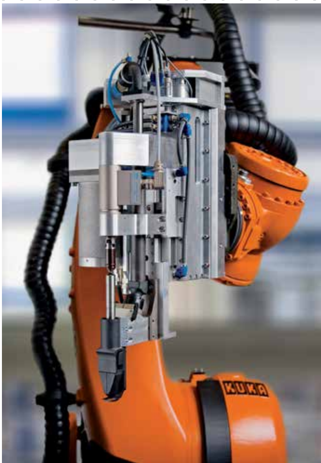
Robot-aided fastening system by Weber Schraubautomaten
