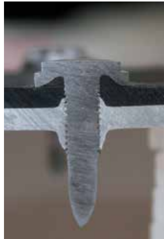
Application example: Composite construction - plastic on aluminium profile
